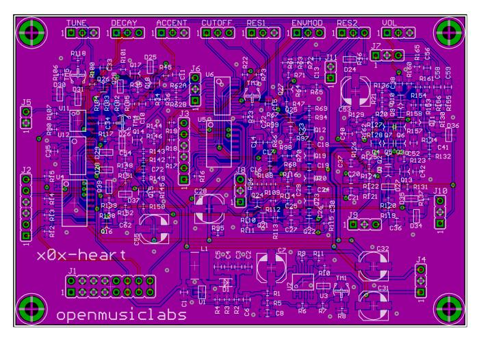
There are 8 headers for potentiometers, and 11 headers for control inputs and outputs. There are also 4 on-board potentiometers for tuning the power-supply, VCO, and VCF. The rest of this document will explain how to tune the x0x-heart, what all of the headers connect to, and how to interface with them. For all headers, pin1 has a square pad, and is labeled with a 1.
